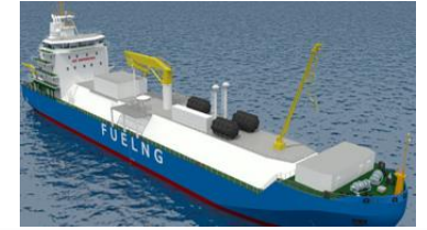
■ FueLNG (Shell/Keppel) ■ 7,500 m3
