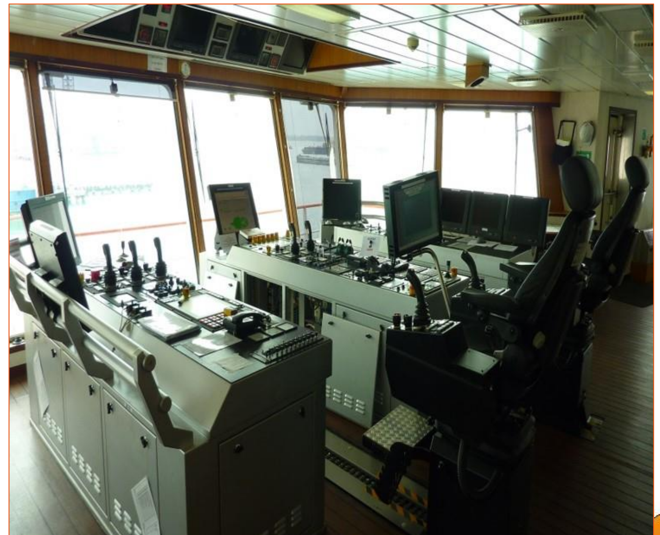
Rear Facing Bridge Control
