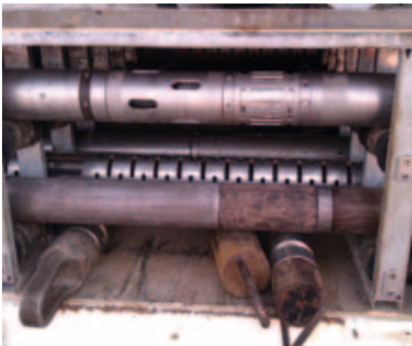
Fig. 5. Geophysical probes: preparation for transportation and insertion into the borehole
