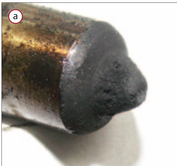
Fig. 2. Coke residue on injector cup in the HPCR system: a) coke residue disintegrating around the fuel outlet orifice, b) crumbling of the coke around the fuel outlet orifice
