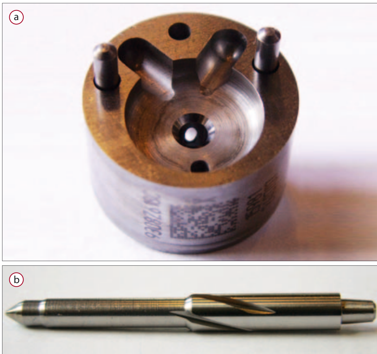
Fig. 5. Viscous, wax seal polymeric organic or amide deposits: a) upper surface of the body of solenoid valve piston controlling the fuel flow, b) injector spray pin
