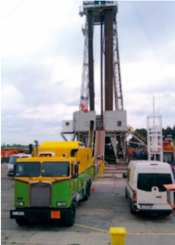
Fig. 4. Well logging in a borehole (truck with equipment for well logging and preparation of the probes before inserting them into the borehole)
