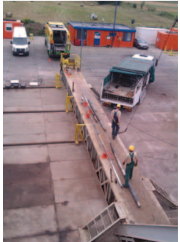
Fig. 4. Well logging in a borehole (truck with equipment for well logging and preparation of the probes before inserting them into the borehole)
