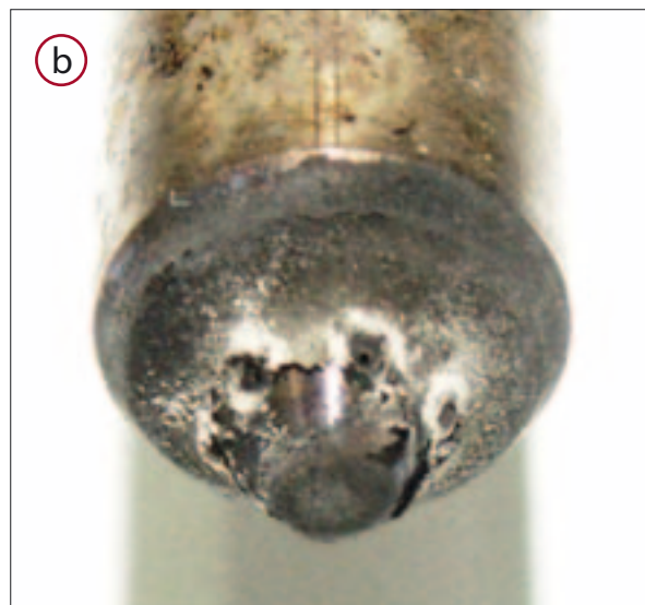
Fig. 2. Coke residue on injector cup in the HPCR system: a) coke residue disintegrating around the fuel outlet orifice, b) crumbling of the coke around the fuel outlet orifice
