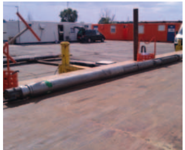
Fig. 5. Geophysical probes: preparation for transportation and insertion into the borehole
