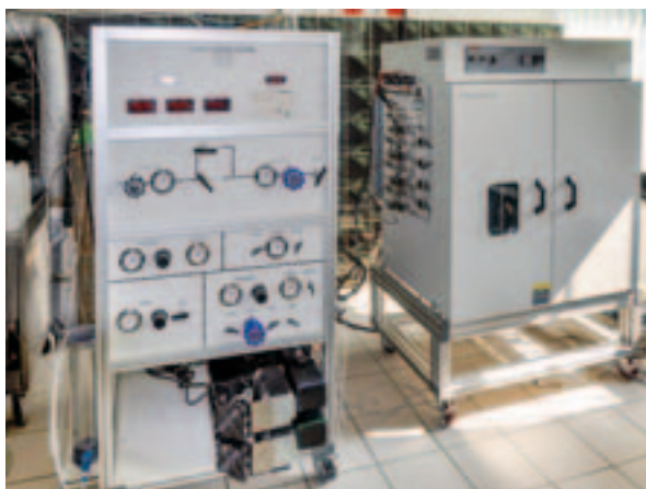
Photo 3. AFS equipment (Acidization Core Flooding System) for testing technological fluids on core samples
