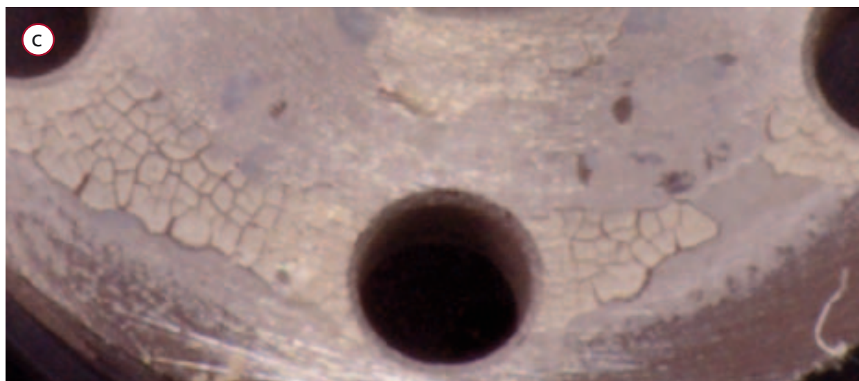
Fig. 4. Deposits of soap which contains metallic ion (mostly sodium or chloride soaps of fatty acids): a) lower surface of solenoid valve piston which controls the fuel flow, b) the view of solenoid valve piston with enlarged surface of the mushroom valve (c)
