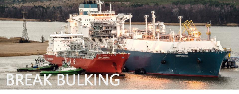
Small modifications enable the transfer of LNG to smallscale vessels enabling regional "virtual pipeline" trade
